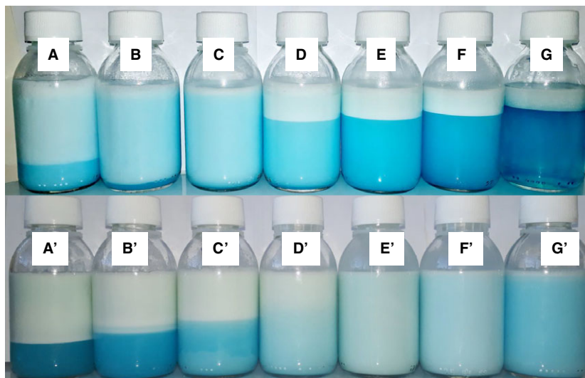
Figure 3 Emulsion of paraffin oil stabilized by a mixture of Tween™ 80/Emulium® Mellifera and Span™ 80/Tefose® 1500 (see Table III).
